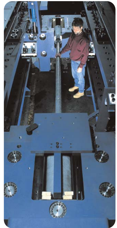
▲ SATEC™ series horizontal testing system with 10 MN (2,250,000 lbf) loading capacity for testing steel cables.
